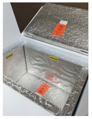
→ The loose skin and lack of rigidity of the back panel indicates the panel has lost its vacuum.
